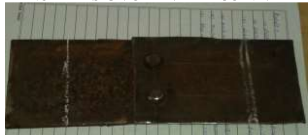
Fig. 2. Riveted joint With adhesive
