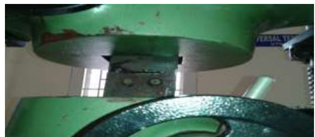
Fig.3. Riveted joint with adhesive under applying load
