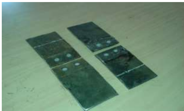
Fig .5. After failure of riveted joints (Both with and without adhesive)
