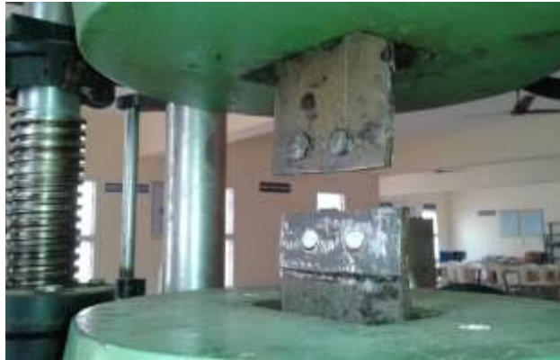
Fig .4. Shear failure of rivet under tensile loading
